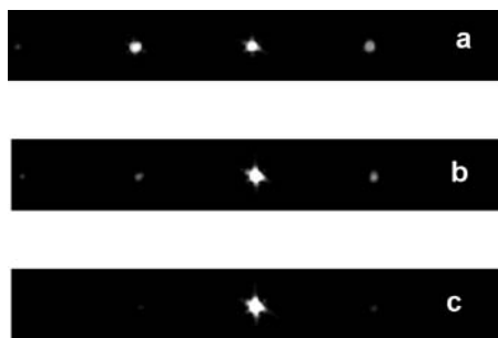
Figure 10. Registered diffraction pattern in planar periodic-planar PDG in the different functioning modes: a - dynamic diffraction 2 ms, 35 V, 7.5Hz bipolar pulse is applied; b - static diffraction, no voltage; c - 1 kHz; 25 V AC voltage is applied.
